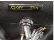
When you wish to push, pull or tow the vehicle, flip the switch under the front seat to TOW & the parking brake will disengage.
